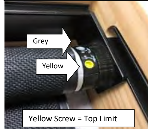
Image 4: Motor on the right side and fabric drops towards the rear of the roller
