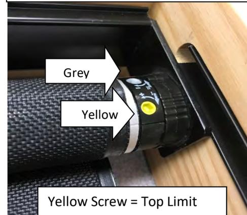
As a general rule for adjusting the shade limit stops, turn either screw counter-clockwise (CCW) to EXTEND the range and turn clock-wise (CW) to SHORTEN the range of the shade, i.e.
