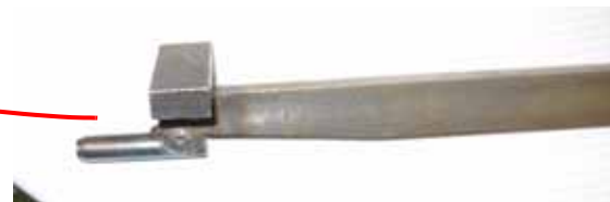
Special Belt Fitting Tool Part No. C00142716
