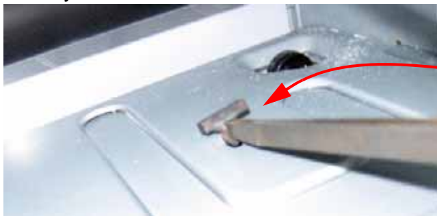
Special Belt Fitting Tool Part No. C00142716
