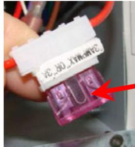
Wire inside fuse should be unbroken. If wire is broken replace.
