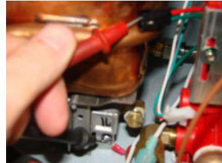
If the motor is still not working verify with a multimeter that it is receiving 12 volts. Do this by using a magnet in proximity of the reed switch to activate the unit. Then place the red lead of the meter on the pin of the black terminal that is attached to the red wire. While placing the black lead of the meter to the metal case. The multimeter should read 12 volts if it does and the motor still isn't functioning when plugged back in the motor is faulty.
