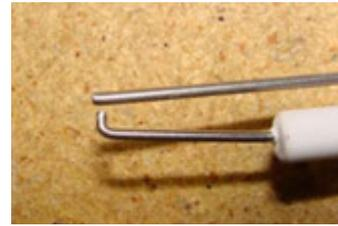
Properly gapped electrode    improperly gapped electrode
