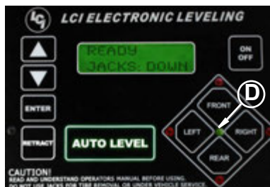
Fig. 3 Touch Panel - Unit Level
