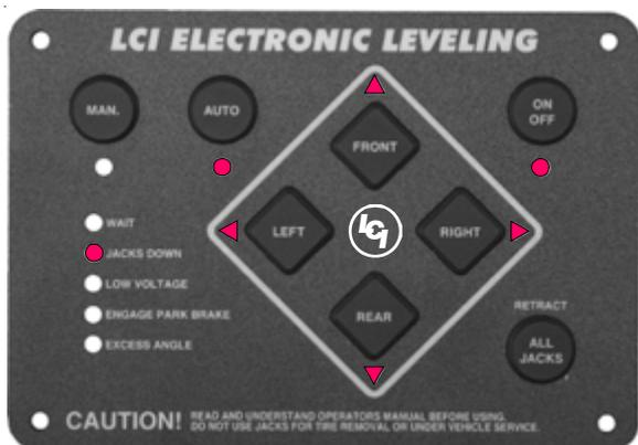
“LCI LOGO” light will go out when coach is initially leveled. The AUTO-LEVELING system will then go through a series of fine-tuning for leveling and the “ARROW” lights will indicate that the coach is leveling itself and which jacks are being activated.
