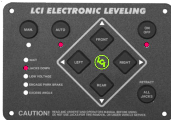
When the system has automatically leveled the coach, the “ON/OFF”, “AUTO”, “JACKS DOWN” and “LCI LOGO” lights will all be illuminated. At this point the touch pad can be turned off.
