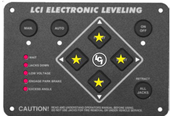
LATCHED ERROR mode is “WAIT,” “JACKS DOWN,” “PARK BRAKE,” “EXCESS SLOPE” AND “LOW VOLTAGE” lights flashing.
