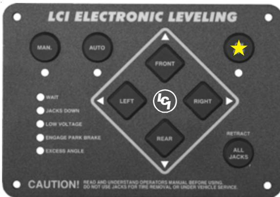
Operator must press “ON/OFF” button ★ to reset operation.
