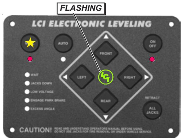
MANUAL LEVELING - Push and hold "MANUAL" button ★ and release. "MANUAL" light will illuminate.
