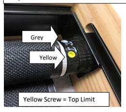
As a general rule for adjusting the shade limit stops, turn either screw counter-clockwise (CCW) to EXTEND the range and turn clock-wise (CW) to SHORTEN the range of the shade, i.e.
