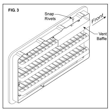
**Important:** The lower vent baffles shown in FIG. 3 may need to be taken out when you stop for the night or if you are going to stay in one spot for a few days, and the outdoor temperature is hot. Under these conditions, more air must pass over the cooling unit in order to maintain good cooling performance.
