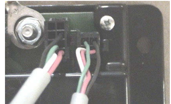
4 & 8 Pin connectors at control module
