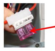
Wire inside fuse should be unbroken. If wire is broken replace.
