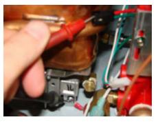
If the motor is still not working verify with a multimeter that it is receiving 12 volts. Do this by using a magnet in proximity of the reed switch to activate the unit. Then place the red lead of the meter on the pin of the black terminal that is attached to the red wire. While placing the black lead of the meter to the metal case. The multimeter should read 12 volts if it does and the motor still isn't functioning when plugged back in the motor is faulty.
