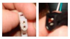
If the motor still doesn't function unplug the motor and verify that the pins on the black terminal properly aligned with the holes on the white terminal
