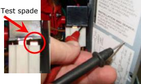
Finally test the relay using a multimeter. The red lead should be placed on the spade closest to the right wall of the unit as pictured. While the black lead can be placed against the metal casing. If the relay is working properly the meter should read near 12 volts.
