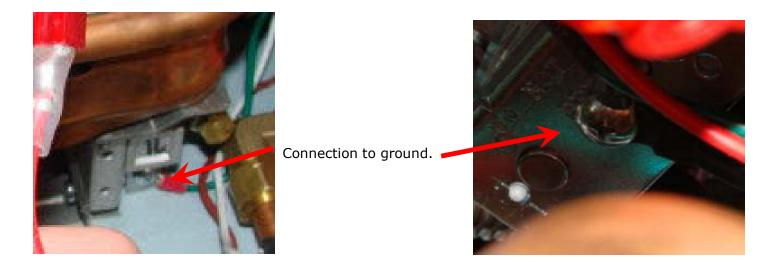
This unit has two ground connections one is below the manifold as seen in the picture to the left. The other is a ground to the valve it's self seen in the picture on the right. Check that these connections are present and not loose.
