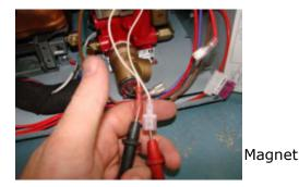
Multimeter leads are placed on separate reed switch leads to test for continuity.
