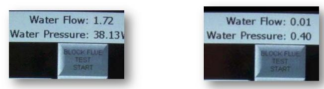
Check the water flow on the tester as pictured above make sure that water flow is below .5 gpm. If it is not shut the valve and make sure the heater turns off if it does not move forward in the trouble shooting guide.
