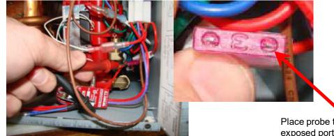
Place probe tip against exposed portion of the fuse
