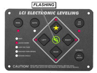
Push "FRONT" button 🖈 and hold. Both FRONT jacks will move at the same time. Hold "FRONT" button until both FRONT jacks touch the ground.
