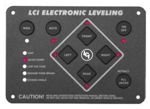
"LCI LOGO" light will go out when coach is initially leveled. The AUTO-LEVELING system will then go through a series of fine-tuning for leveling and the "ARROW" lights will indicate that the coach is leveling itself and which jacks are being activated.
