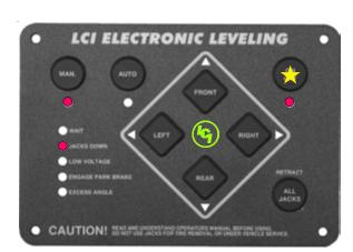
MANUALLY LEVEL the coach. Turn the TOUCH PAD "OFF" . Turn the TOUCH PAD "ON" again. This readies the TOUCH PAD for reprogramming the LEVEL ZERO POINT.
