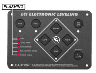
LATCHED ERROR mode is "WAIT," "JACKS DOWN," "PARK BRAKE," "EXCESS SLOPE" AND "LOW VOLTAGE" lights flashing.
