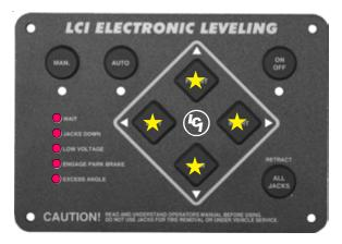
Retract time over 90 seconds in auto retract. This is the only LATCHED ERROR MODE. All revisions prior to "G" controllers treat this error as regular ERROR mode. To RESET, push all 4 diamond-shaped jack buttons at the same time.
