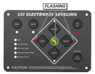
If an issue involving the system occurs, the TOUCH PAD will register an ERROR MODE alert, indicated by the "LCI LOGO" and the "LEFT" and "RIGHT" arrow lights flashing.
