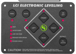
The TOUCH PAD will sound an alarm and the TOUCH PAD will flash all lights for either of two possible reasons; (1) A "RETRACT" hose is leaking or (2) the pressure holding the retracted jacks falls below 1500 psi.
