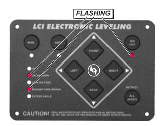
If TOUCH PAD and CONTROLLER lose communication for more than 5 seconds, the TOUCH PAD will flash the "JACKS DOWN", "ENGAGE PARK BRAKE", and "ON/OFF" lights. Turn off ignition and check that TOUCH PAD and CONTROLLER are securely connected.
