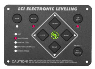
When the system has automatically leveled the coach, the "ON/OFF", "AUTO", "JACKS DOWN" and "LCI LOGO" lights will all be illuminated. At this point the touch pad can be turned off.
