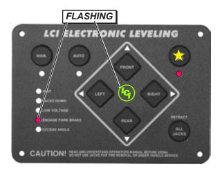
Push "ON/OFF" button . "ON/OFF" light illuminates; "LCI LOGO" light flashes. If PARK-ING BRAKE is not engaged, "PARKING BRAKE" light will flash. Engage PARKING BRAKE.
