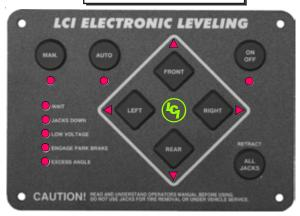
The system ALARM will sound and all TOUCH PAD lights will flash if the PARKING BRAKE is release and at least one (1) jack is not fully retracted or if the ignition is in the "RUN" position and the jacks are down. The system will perform an automatic retract.
