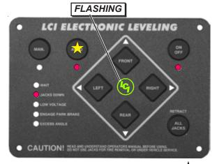
AUTO-LEVELING - Push "AUTO" button and release. "AUTO" light will illuminate and the "LCI LOGO" light will flash when pump begins to run. "JACKS DOWN" light will illuminate indicating the jacks are moving. DO NOT TOUCH PAD DURING THIS PROCESS.
