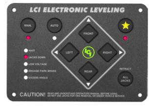
When the "LCI LOGO" stops flashing and simply stays on, the coach is level. The TOUCH PAD can now be turned off by pushing the "ON/OFF" button ...
