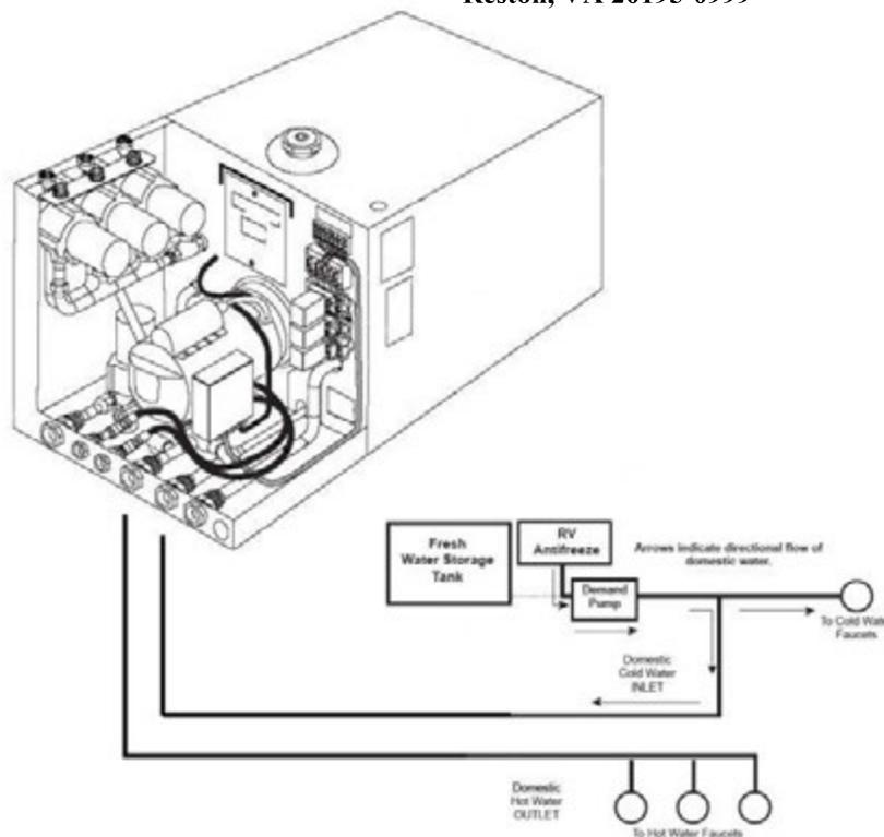
5. Open and close all interior and exterior water faucets, one at a time, until only pure RV Antifreeze is present. Perform this procedure for both the hot and cold faucets.
