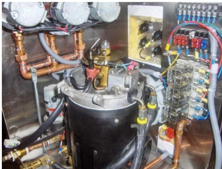
1. Using Pliers loosen the constant tension clamps securing the fuel lines to the diesel burner, and slide away from the burner.
