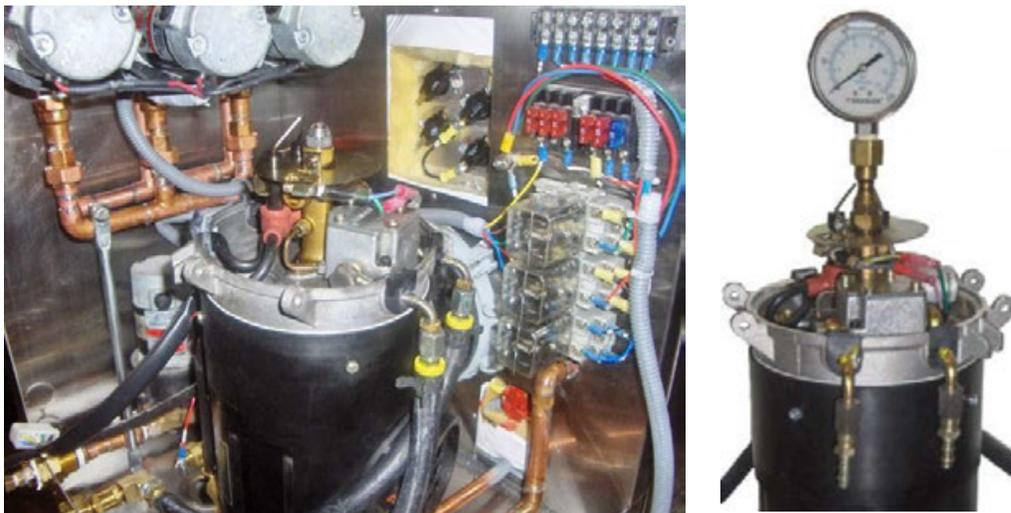
1. Remove the Diesel Burner and install the Fuel Pressure Gauge .
