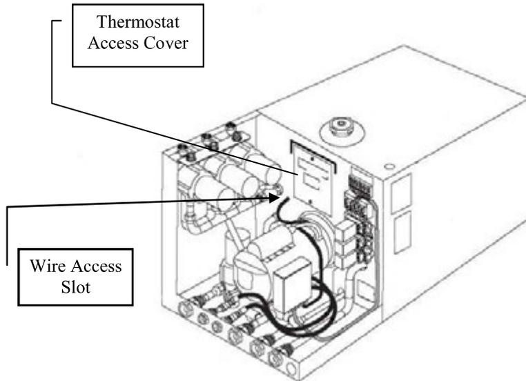
1. Using a Phillips head Screw Driver loosen the screws securing the thermostat access cover in place, and remove the thermostat access cover.
