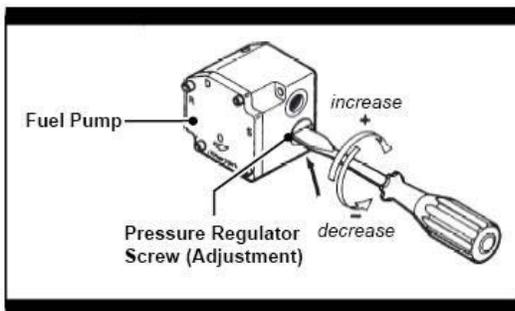
1. Once the fuel solenoid has been activated, and the fuel pressure gauge is registering a pressure, the fuel pressure can be adjusted. To increase the fuel pressure turn the pressure adjustment screw clockwise, and to reduce the fuel pressure, turn the pressure adjustment screw counter clockwise.
