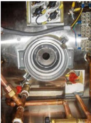
1. Remove the combustion chamber by pulling it straight out, approximately 16 inches.
