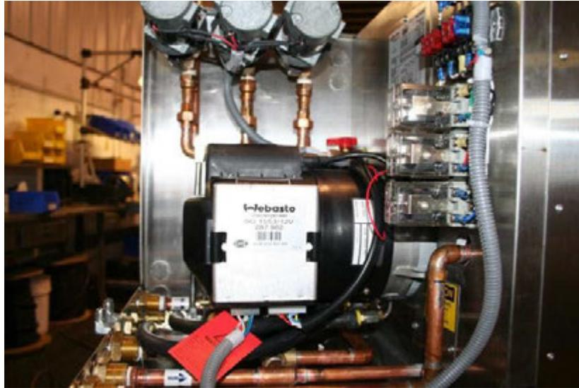
NOTE: The Diesel Burner's Controller might have to be mounted onto the side of the diesel burner, before the plugs are inserted into the control unit, otherwise it might not be possible to mount the control unit.
