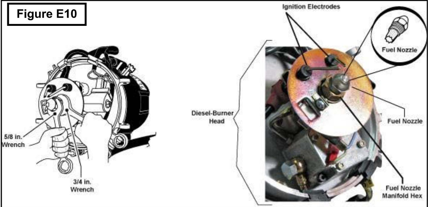
1. Use a 3/4 in. wrench to hold the fuel nozzle manifold hex, while loosening the fuel nozzle with a 5/8 in. wrench and remove.
