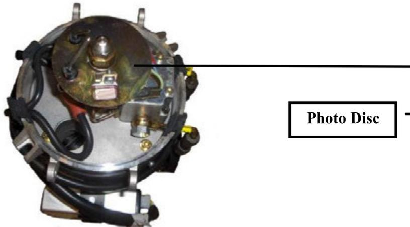
1. If the photo disc is not free floating, the electrode clamp bolt has been over-tightened, and has bent the electrode clamp. Using a 10mm socket remove the electrode clamp, and re-straighten.
