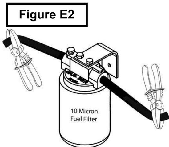
3. Replace fuel filter, with proper replacement canister.
