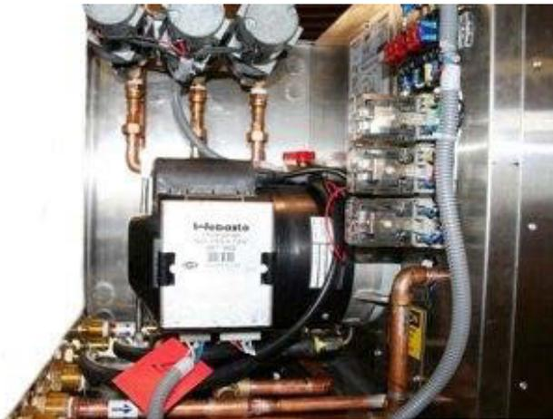
1. Locate the Diesel-Burner's Controller and disconnect both plugs.
